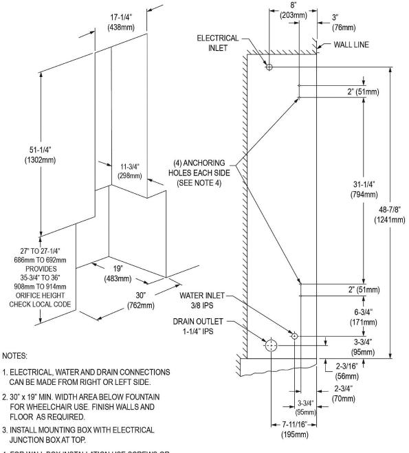
4. FOR WALL BOX INSTALLATION USE SCREWS OR BOLTS (MIN. OF 8) THRU HOLES OR KNOCK-OUTS PROVIDED ON EACH SIDE. (SCREWS OR BOLTS TO BE FURNISHED BY INSTALLER).
