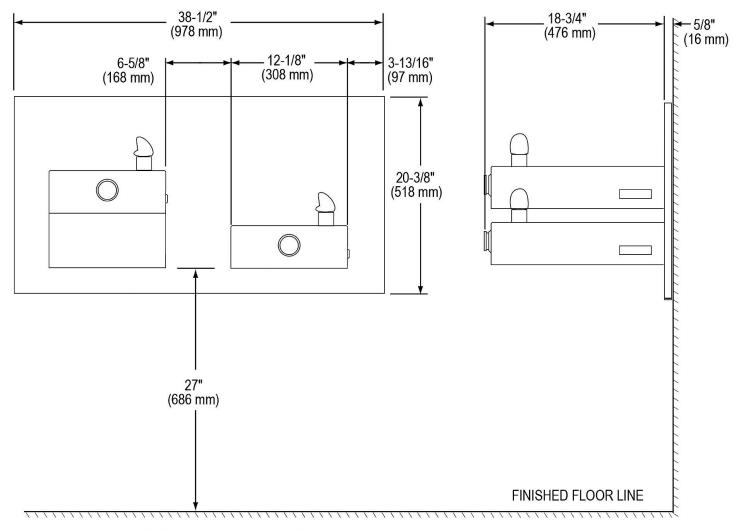
\*A.D.A. Compliant (24" [610mm] for Child A.D.A.). Adjust other measurements accordingly
