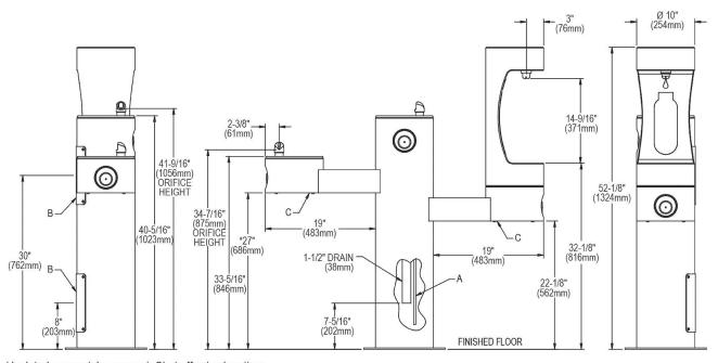
A = 3/8" O.D. Unplated copper tube connect. Shut off valve by others. B = Access panel(8" x 10").
