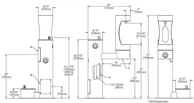
A = 3/8" O.D. Unplated copper tube connect. Shut off valve by others.
