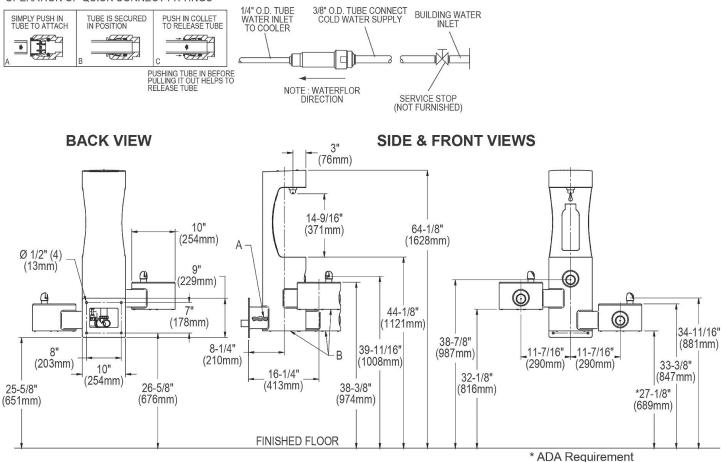
A = 3/8" O.D. UNPLATED COPPER TUBE CONNECT - SHUT OFF VALVE BY OTHERS
