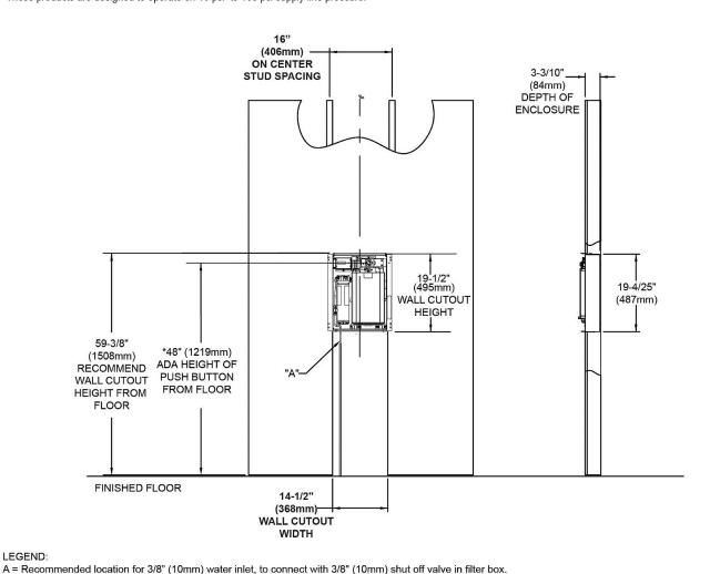
\*Height to top of wall cutout will need to be less than the recommended 59-3/8" (1508mm) height to meet the ADA requirement for the push button location of 48" (1219mm).
