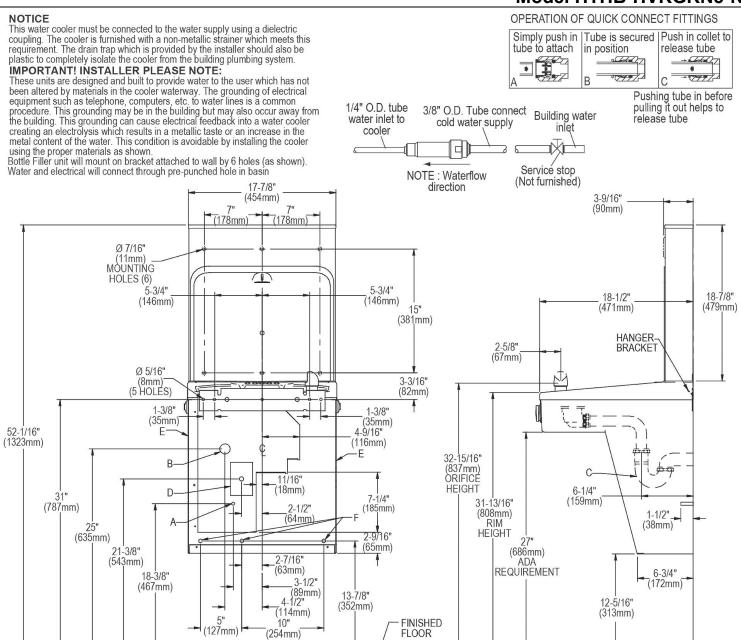
A = Recommended Water Supply location. Shut-off Valve (not furnished) to accept 3/8" O.D. unplated copper tube. Up to 3" (76mm) maximum out from wall. B = Recommended Waste Outlet location. To accommodate 1-1/4" nominal drain. Drain stub 2" (51mm) out from wall.
