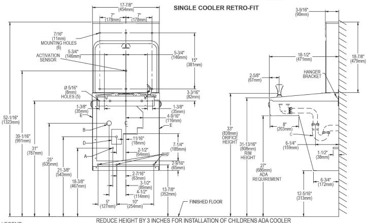
A = Recommended Water Supply location. Shut-off Valve (not furnished) to accept 3/8" O.D. unplated copper tube. Up to 3" (76mm) maximum out from wall.
