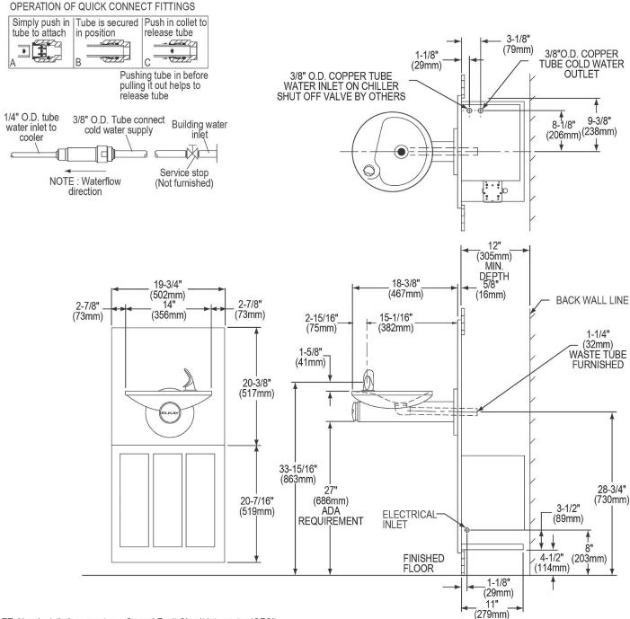
NOTE: New installations must use Ground Fault Circuit Interrupter (GFCI).
