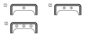
1-1/4" (32mm) Diameter Faucet Holes For 1 and 2 Hole Models 1-1/2" (38mm) Diameter Faucet Holes For 3 Hole Model Faucet Holes on 4" (102 mm) Centers
