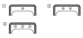
1-1/4" (32mm) Diameter Faucet Holes For 1 and 2 Hole Models 1-1/2" (38mm) Diameter Faucet Holes For 3 Hole Model Faucet Holes on 4" (102 mm) Centers
