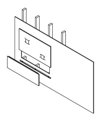
Includes the access panel and L-bracket for mounting. The access panel has a tab along the top which secures behind the fountain back panel. L-bracket is mounted to the wall. Access panel is secured to L-bracket with screws.
