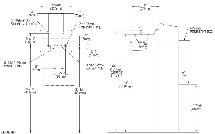
A: Recommended water supply location, 3/8" O.D. unplated copper tube connect stub
