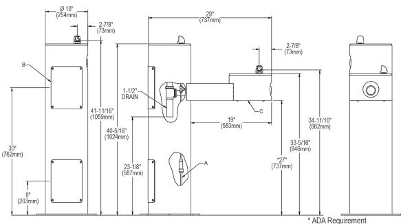
A = 3/8" O.D. Unplated copper tube connect
