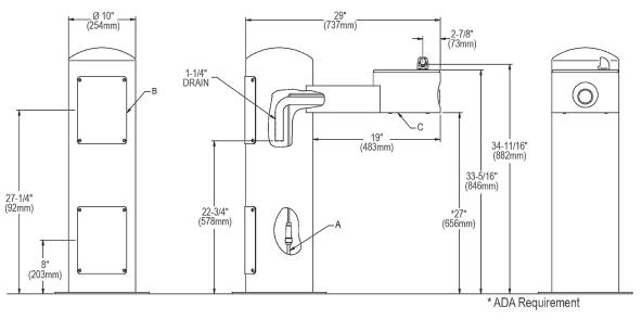
A = 3/8" O.D. Unplated copper tube connect
