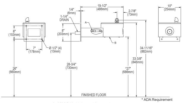
A = 3/8" O.D. Unplated copper tube connect
