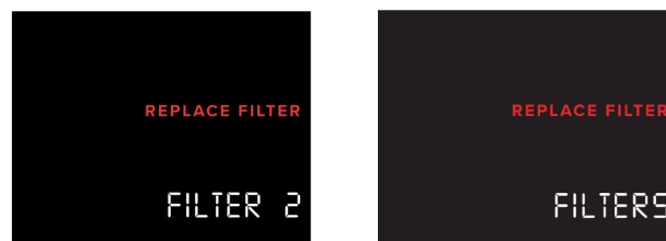
FILTER 2 EXPIRED (Contaminant filter)
