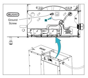
5. Connect the black wire (B) to supply voltage HOT and connect the white wire (C) to neutral line.
