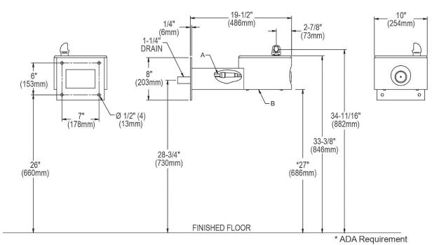
A = 3/8" O.D. Unplated copper tube connect shut off valve by others
