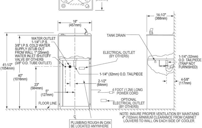
NOTE: New installations must use Ground Fault Circuit Interrupter (GFCI). It is highly recommended that the circuit be dedicated and the load protection be
