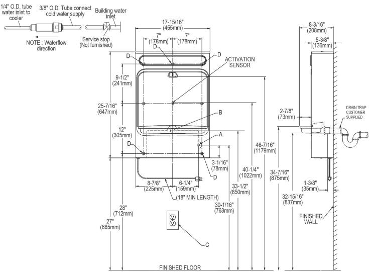
A = Recommended water supply location; 1/2" I.P.S. maximum pipe size. Service stop valve not furnished.
