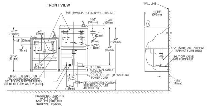
NOTE: New installations must use Ground Fault Circuit Interrupter (GFCI).
