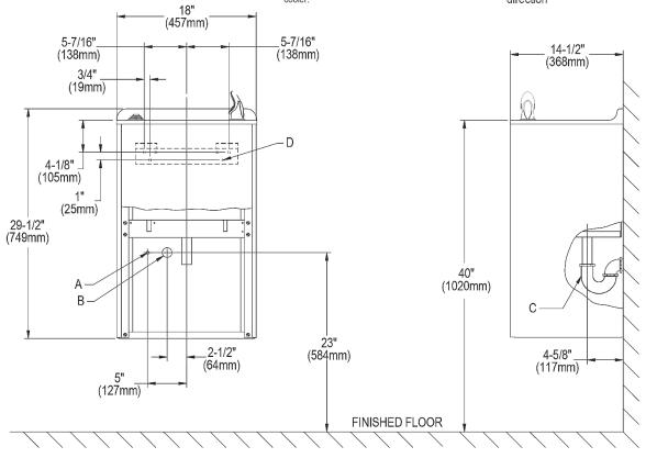
A = Recommended water supply location 3/8" O.D. unplated copper tube connect stub 1-1/2" (38mm) out from wall shut off by others.
