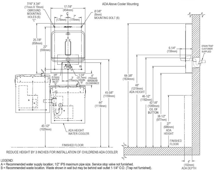
C = 7/16" X 3/4" Obround mounting holes for fastening backplate to wall. NOTE: New Installations Must Use Ground Fault Circuit Interrupter (GFCI). It is highly recommended that the circuit be dedicated and the load protection be sized for 20 amps.
