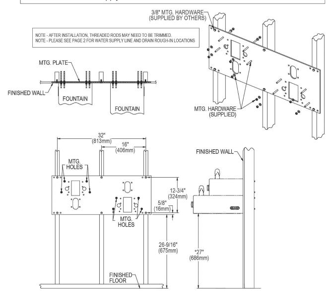
\*ADA REQUIREMENT NOTE - AFTER INSTALLATION, THREADED RODS MAY NEED TO BE TRIMMED
