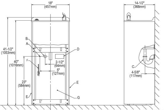
**LEGEND** A = Recommended water supply location 3/8" O.D. unplated copper tube connect stub out 1-1/2" (38mm) from wall shut off by others.
