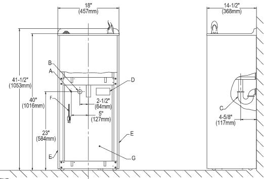
A = Recommended water supply location 3/8" O.D. unplated copper tube connect stub out 1-1/2" (38mm) from wall shut off by others. B = Recommended location for waste outlet 1-1/4" O.D. drain. C = 1-1/4" Trap not furnished.
