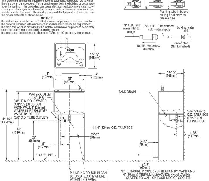
NOTE: New installations must use Ground Fault Circuit Interrupter (GFCI). It is highly recommended that the circuit be dedicated and the load protection be
