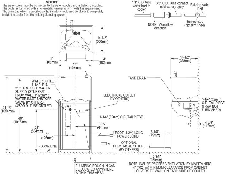
NOTE: New installations must use Ground Fault Circuit Interrupter (GFCI).
