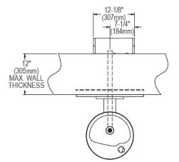
WARNING: The free-resistant box must be installed on an interior heated wall where the temperature does not drop below 50° F (10° C). The front of the box must have unobstructed air flow. Failure to maintain the interior wall temperature and the inside of the freeze resistant box above 50° F (10° C) can result in damage to the box which could result in unrestricted
