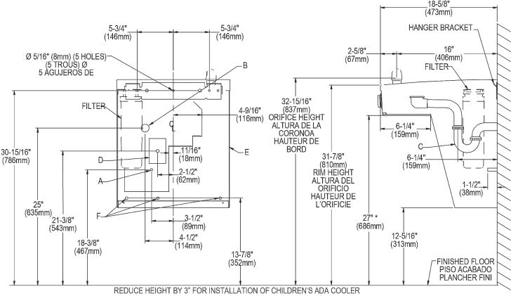
A = Recommended Water Supply location. Shut-off Valve (not furnished) to accept 3/8" O.D. unplated copper tube. Up to 3" (38mm) maximum out from wall. B = Recommended Waste Outlet location. To accommodate 1-1/4" nominal drain. Drain stub 2" (51mm) out from wall.
