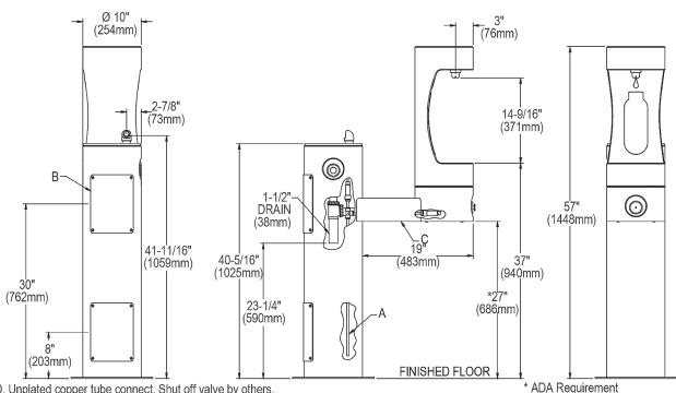
A = 3/8" O.D. Unplated copper tube connect. Shut off valve by others. B = Access panel(8" x 10").
