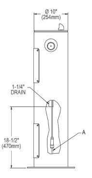
A = 3/8" O.D. UNPLATED COPPER TUBE CONNECT SHUT OFF VALVE BY OTHERS B = ACCESS PANEL (8" x 10")
