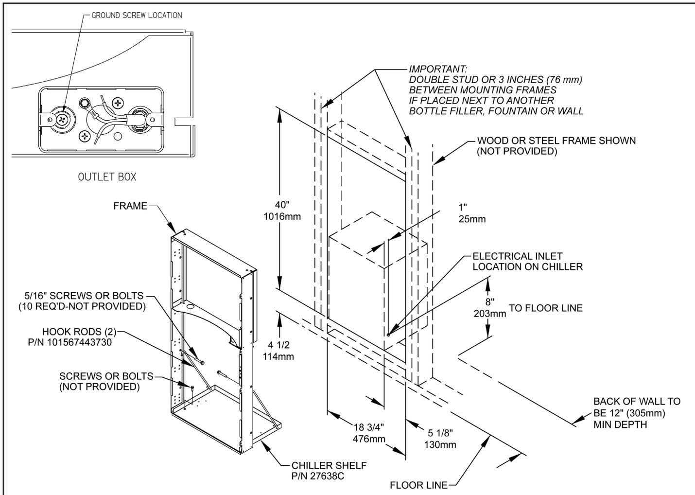
1. Cut a square rectangular wall opening 18 3/4" (476mm) W x 40" (1016mm) H and 4 1/2" (114mm) above the floor line. These dimensions are required to obtain proper rim and bubbler heights for compliance with ANSI standard A117.1.
