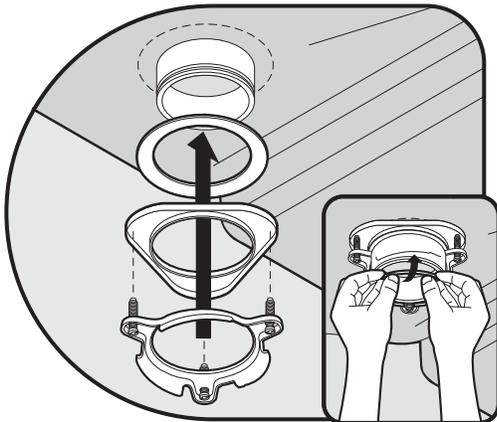
2. Disassemble Quick Lock® mounting assembly components provided with disposer (1, 2, 3, 4, 5, 6)
